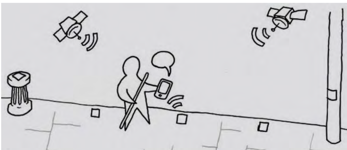
Figure 21 - RFID and GPS technology as a navigation aid to those with visual difficulties (Atkin, 2010)
