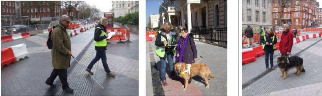
Figure 12.8: Testing of 800mm wide corduroy paving on Exhibition Road in London (MVA Concultancy, 2011a)
