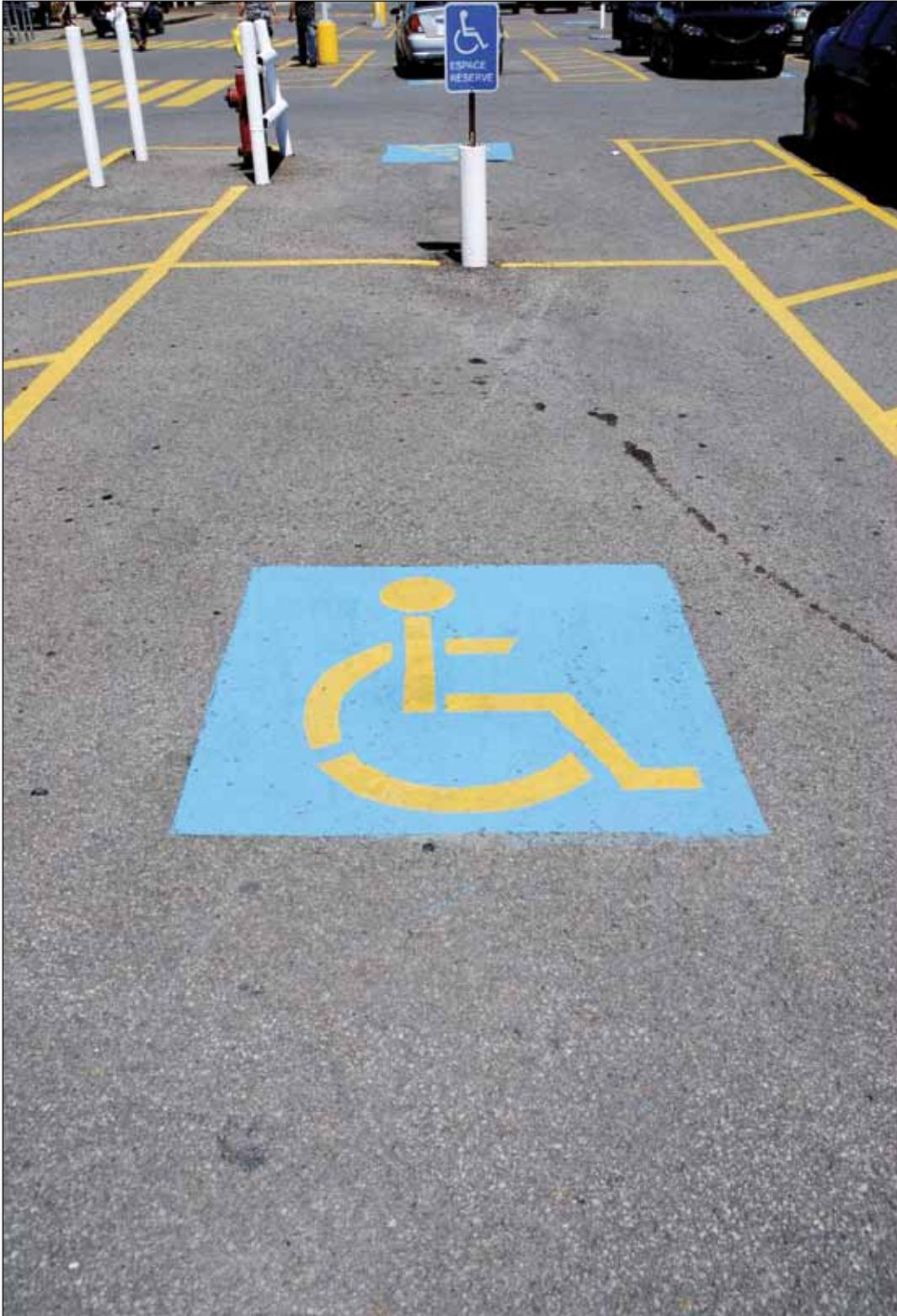
**Image 1.4** Example of insufficient accessible parking spaces. Please note the lack of a post-mounted sign with the international symbol of access fixed to it and the lack of dropped kerbs.
