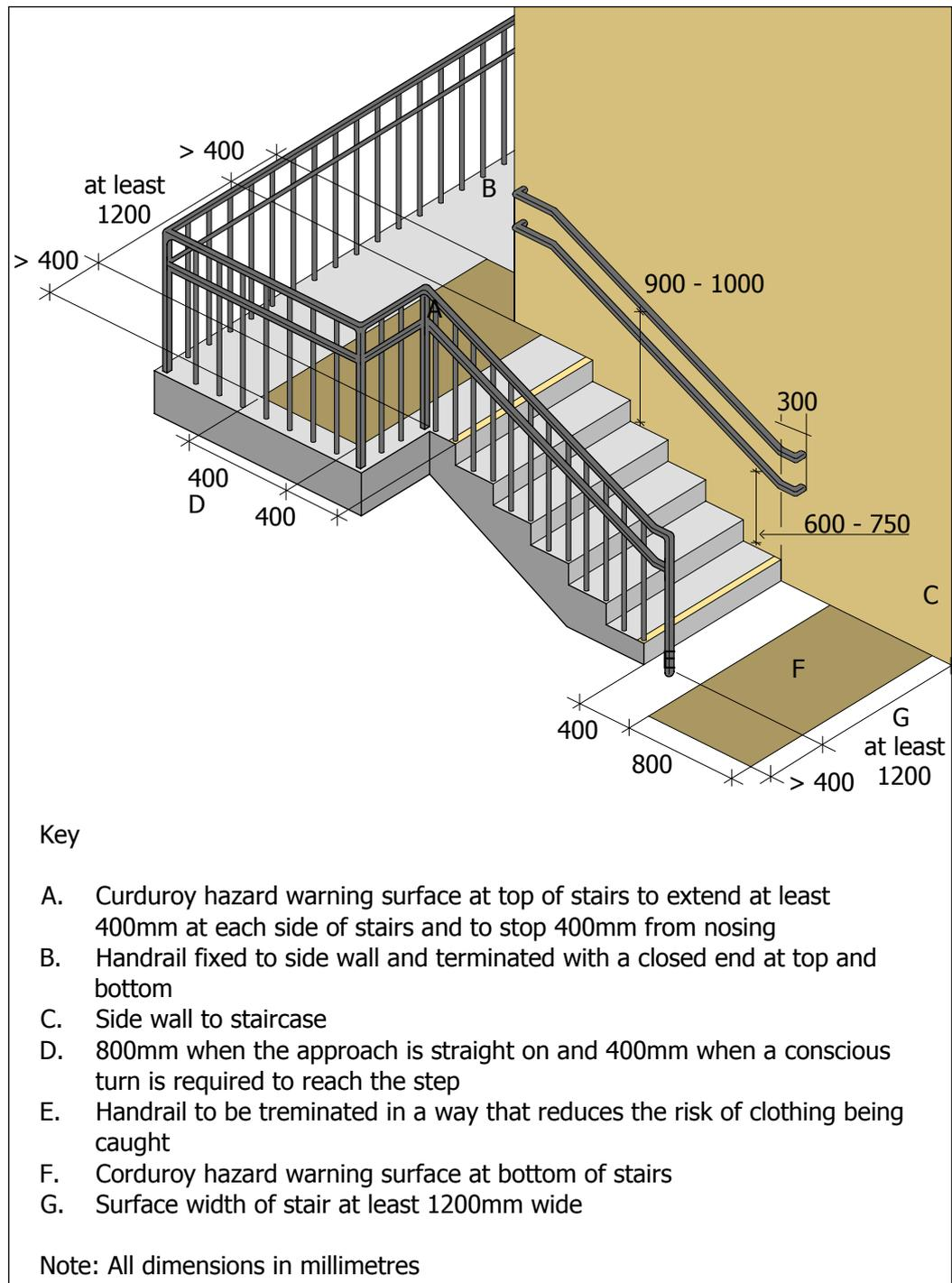
Hazard warning surfacing should not generally be used on intermediate landings as this can give the false impression that the end of a flight has been reached. The exception to this is if the stepped route can be joined at intermediate landing level from another direction, such as via a doorway or adjoining path. Also, if an
