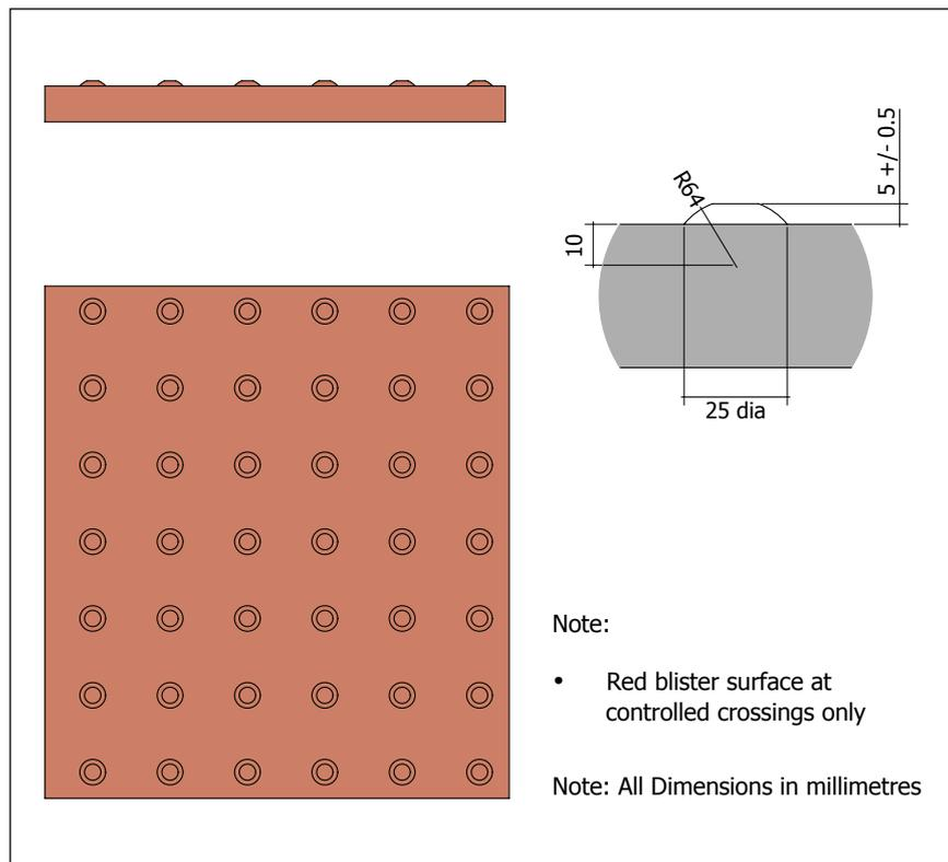
A red blister surface should be used at controlled crossings only. A buff blister surface should be used at uncontrolled crossings. In all cases, the surrounding paving surface should visually contrast with the blister paving to provide visual indication of the extent of the pavement.
