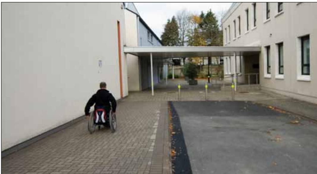
Where the clear width of an access route is less than 2000mm, passing places should be provided. Passing places should be 2000mm wide x 2500mm long, at a reasonable frequency and located within sight of another passing place, subject to a maximum distance of 25m. This will allow groups of people to pass each other, particularly on busy routes. On long routes, level resting places should be provided off the path of travel at intervals of no more than 30 metres.
