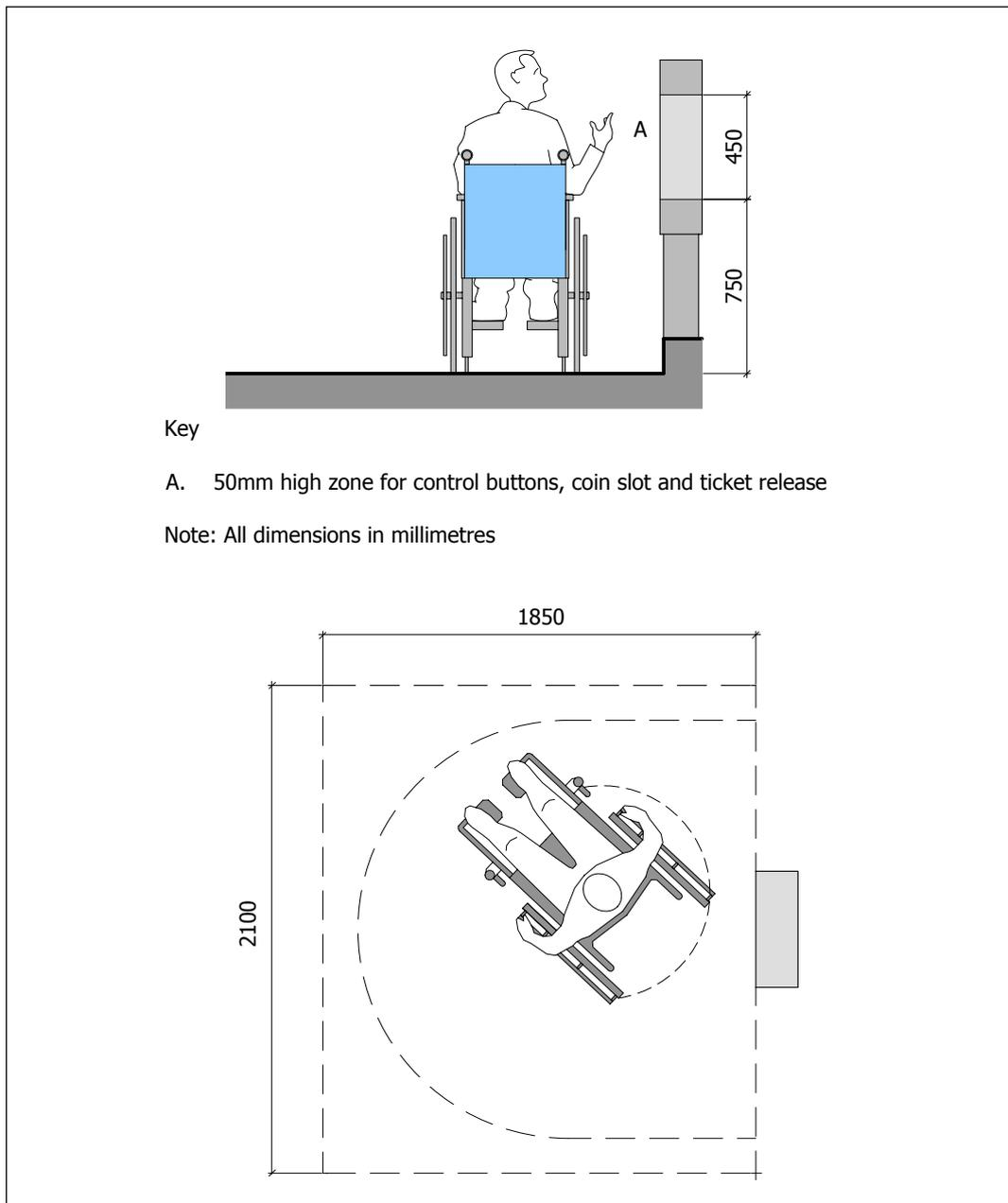
If ticket machines are mounted on a plinth, the edges of the plinth should not project beyond the face of the machine as this can make approach difficult for wheelchair users.
