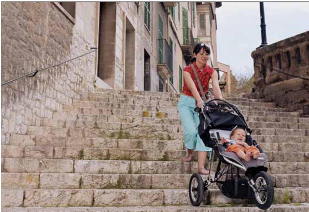
Where the change in level is such as to require steps or a ramp, both should be provided to meet the needs of all building users.
