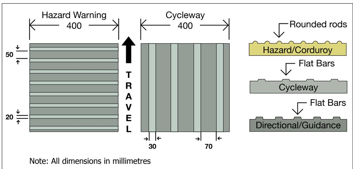
**Image 1.41 and Image 1.42** Note that the tactile paving is aligned longitudinally for the cycleway section (right-hand side) and transversely for the pedestrian section (left-hand side).
