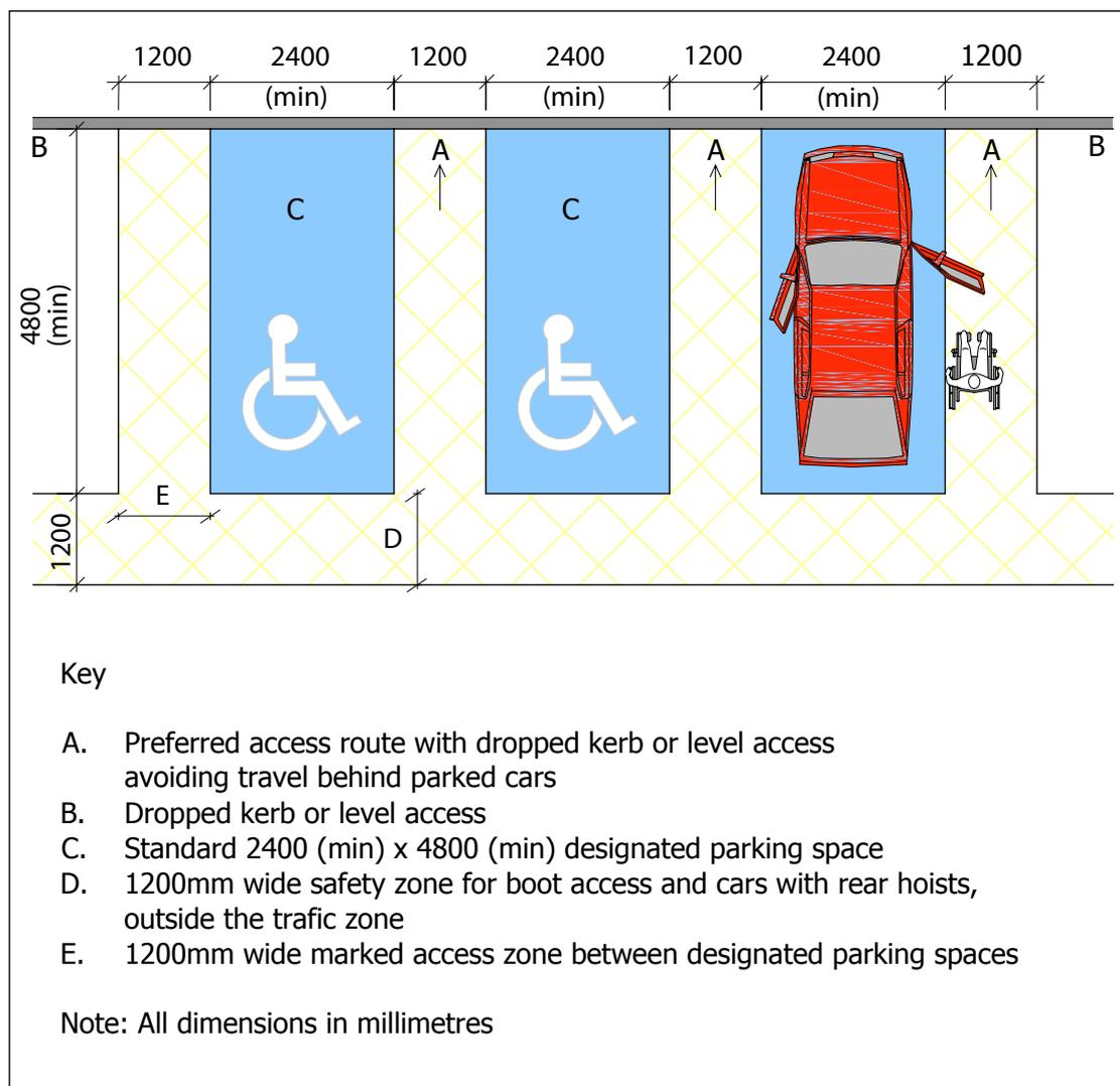
(Extract from Department of Transport, UK 'Traffic Signs Manual'). Off-street (perpendicular) designated parking spaces should be 2400mm (min) wide and 4800mm (min) long, with a layout based on **Figure 1.3**. Each space should have a recommended 1200mm clear access zone to both sides and the end of the space.
