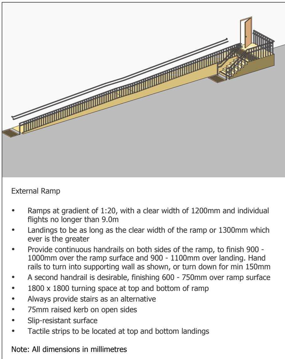
Where the topography of the site is such that changes in level are unavoidable, access routes should be designed for ease of access. They should be understandable, useable, and offer choice.
