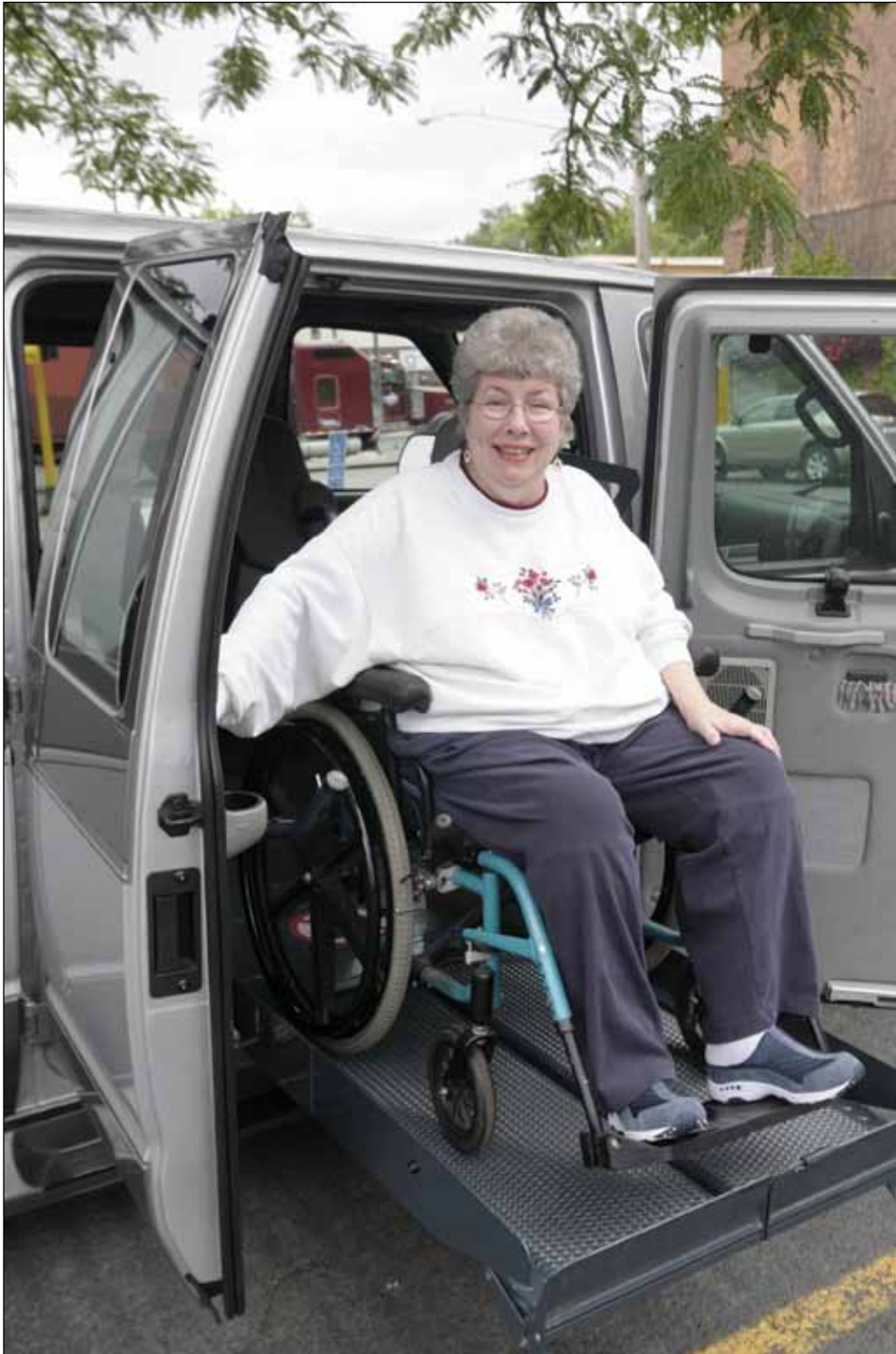
Image 1.2 Example of the importance of providing space to the side of an accessible car parking space.
