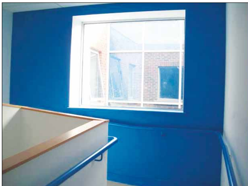
Image 4.4 Example of wall painted as a wayfinding guide for people with visual difficulties.
