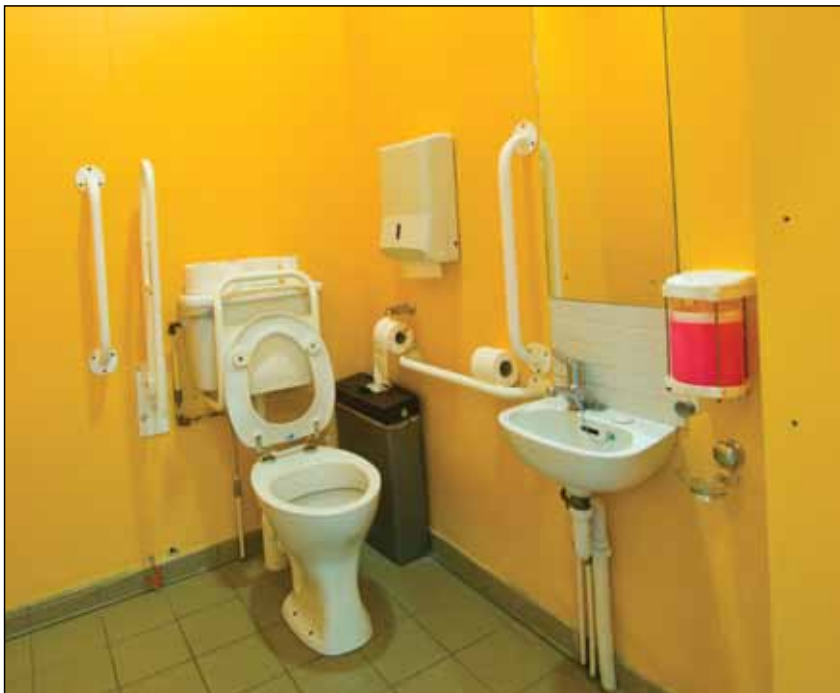
Image 5.8 Example of unisex accessible toilet – left-handed transfer.
