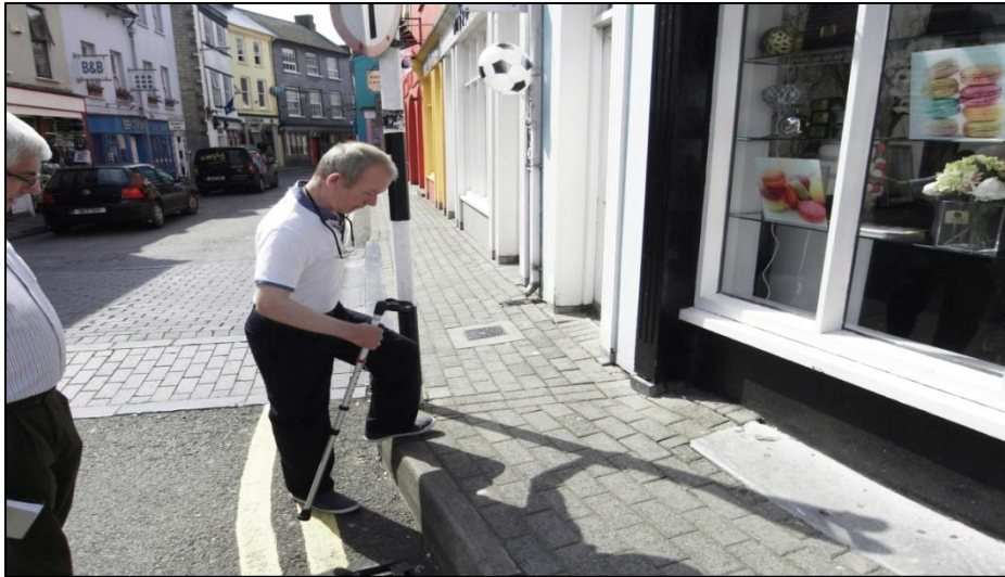
Image 2.3 High kerbing in a town forcing an older adult with mobility issues to pull himself onto the footpath with the assistance of a road sign.
