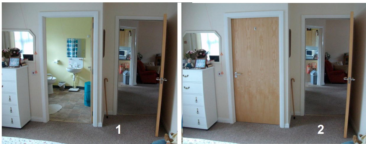
Figure 39 – Image showing colour contrast between floors and walls and between walls and internal doors
