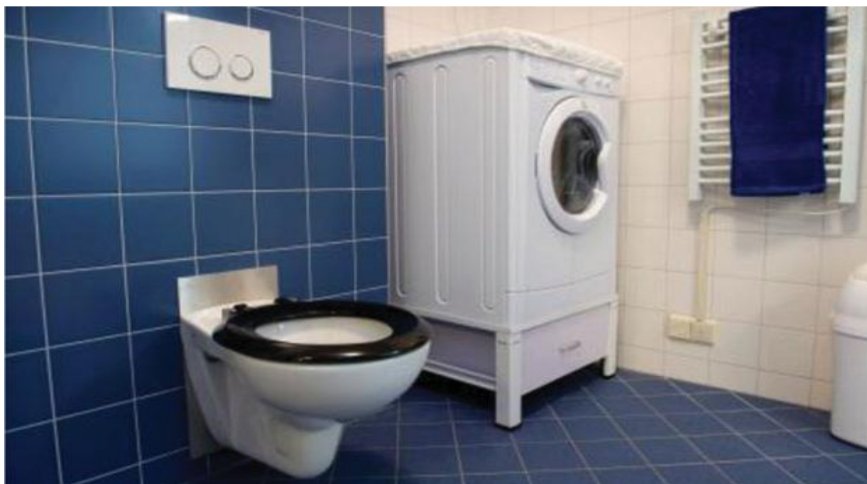
Figure 26 – view to bathroom showing colour contrast between WC and wall (van Hoof et al., 2013)
