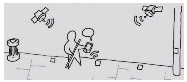
**Figure 21** - RFID and GPS technology as a navigation aid to those with visual difficulties (Atkin, 2010) Willis describes an RFID information grid to assist people with a visual impairment with navigation and wayfinding in a campus setting (Willis and Helal, 2005). This involves the
