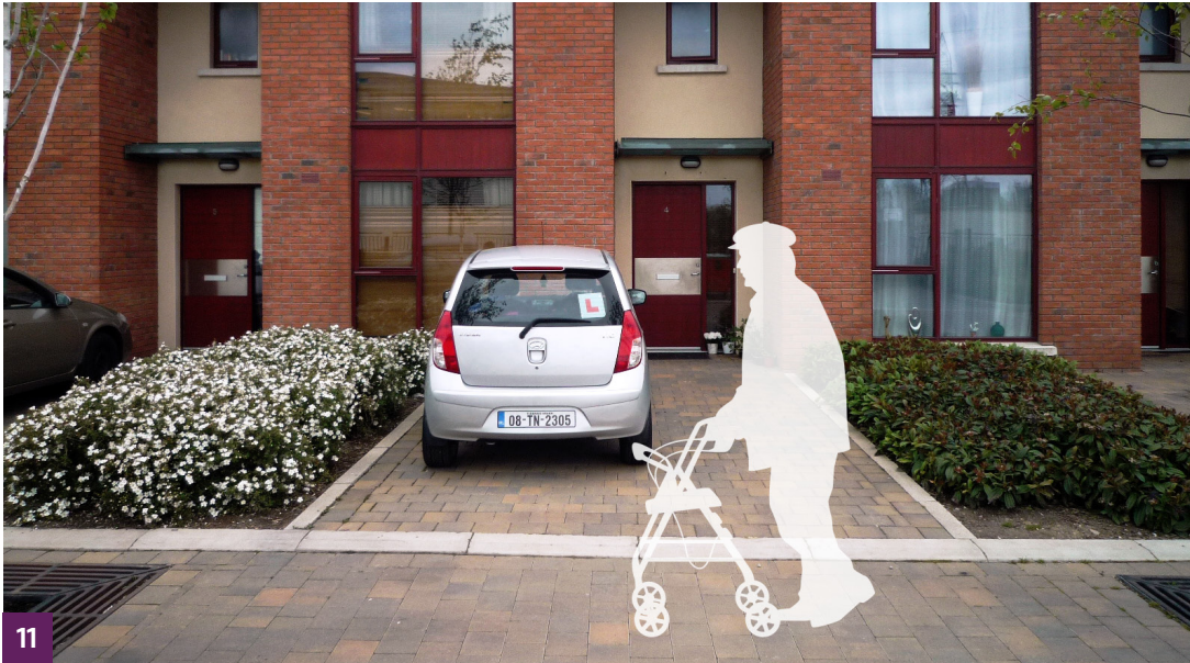
Footpath to front door located adjacent to parking space, creating a flexible space for everyone to use.
