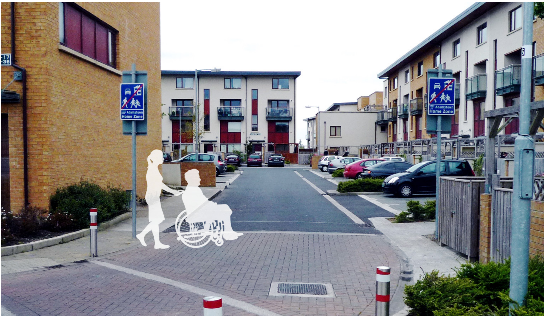
The parking area is clearly designated as a shared surface area.
