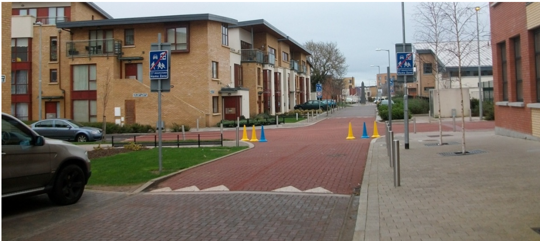
Figure 12.5: This transition zone alerts drivers to the fact that they are entering or leaving the Home Zone, yet on the footpath to the right there is not such notification.
